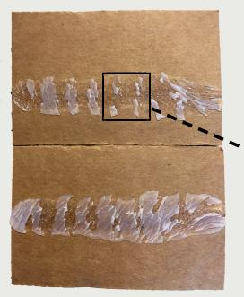
Cold resistance failure occurs when the glued substrate has been exposed to low temperatures below that of the adhesive service temperature. Failure does not occur during the manufacturing process, but rather during transport or storage.
