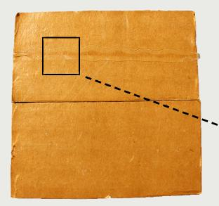
Poor adhesion occurs simply when the adhesive is unable adhere to the substrate. This failure may be due to using the wrong type of adhesive for the substrate and/or the substrate may have a difficult-to-bond coating.
