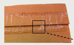
Chewing gum failure occurs when the adhesive is too hot, there is too much adhesive applied, or the adhesive is too slow to form a bond.
