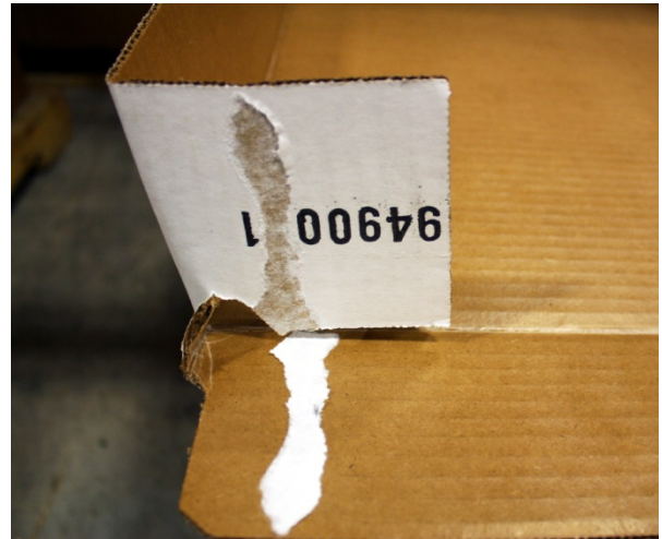
The newly implemented adhesive was able to penetrate through the wax to reach the corrugate and form a 100%, full fiber-tearing bond for maximum adhesion.
