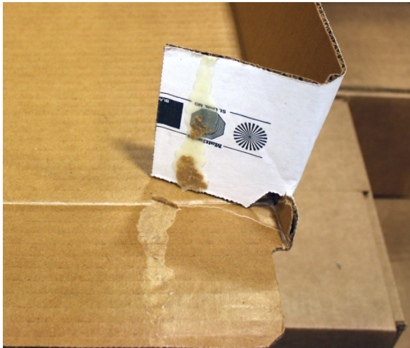
The initial adhesive was unable to penetrate through the wax corrugated. This resulted in a superficial bond, causing pop-opens upon cooling.
